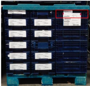
incomplete SLC on top level
